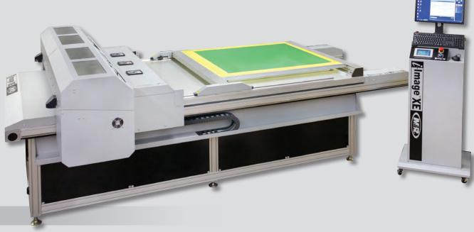
• i-Image XE models can generate and expose full-size T-Shirt images in less than a minute
