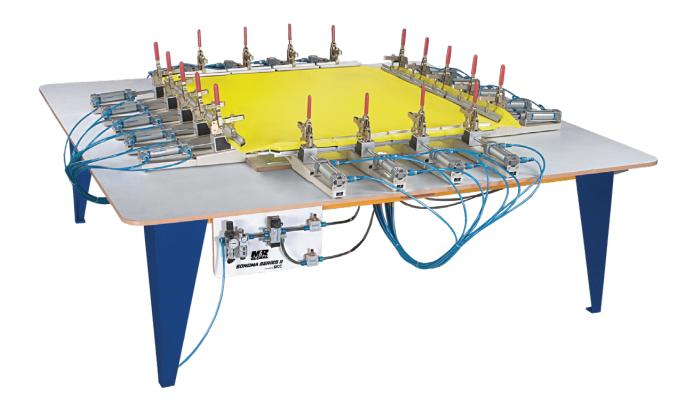
Present days' screen printing demands high density, high resolution and accurate outputs. Fabric tension plays an important part in achieving the desired results. M&R's Sonoma Series II is specially designed to achieve perfect fabric tension.
