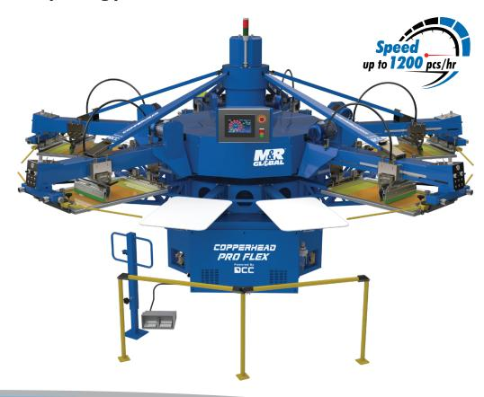
M&R Global DCC 's Copperhead Pro Flex ™ presses are the benchmark in automatic screen printing presses, combining highest quality components, leading-class craftsmanship and high-speed production to create an outstanding press at an affordable price. An electric indexing system enables extremely smooth and quiet operation. The included, innovative squeegee pressure equalizer system with regulators on each printhead speeds setup and ensures uniform ink deposit for excellent print quality.
